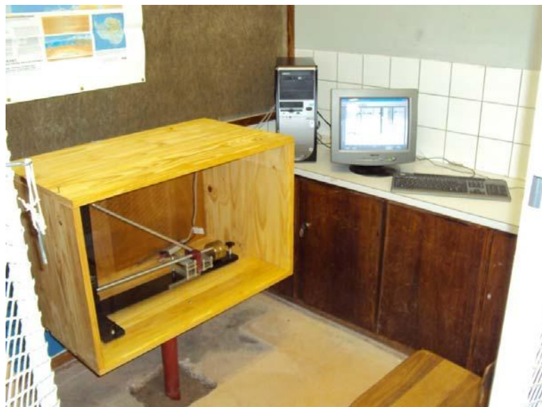
Figure 14. A seismometer at Etosha Secondary School.
